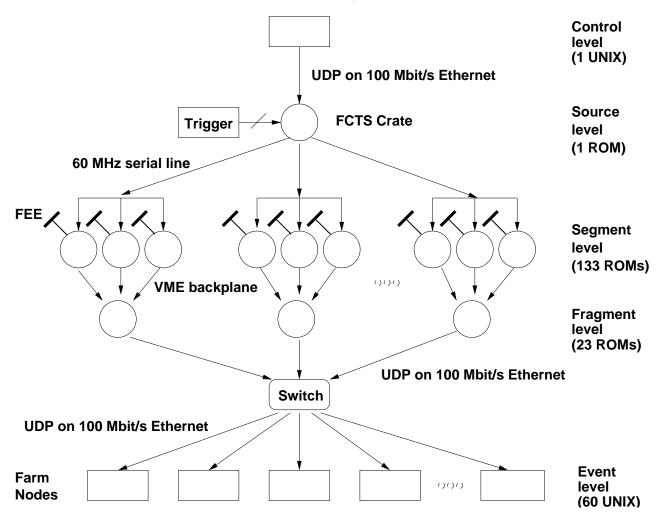
• ODF able to receive 1 Mbyte input data @ L1 trigger rate of 4 kHz, filter it to about 24 kbytes of event data
